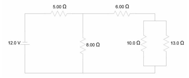
(a) Calculate the total resistance of the circuit.
