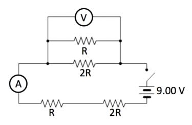
(a) When the switch is closed, calculate the current displayed by ammeter A.
